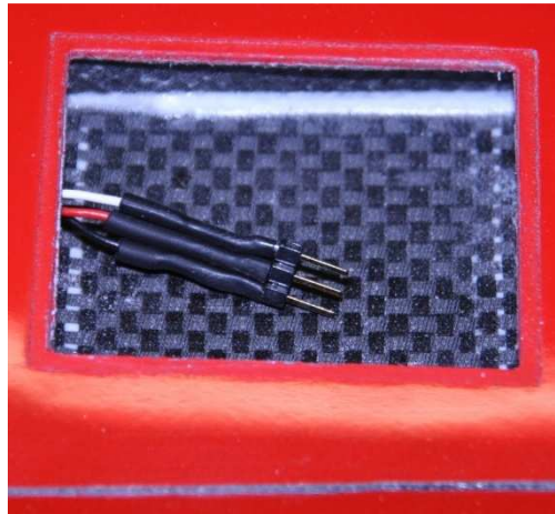
Picture 11: The cables of servos and septa of servos
