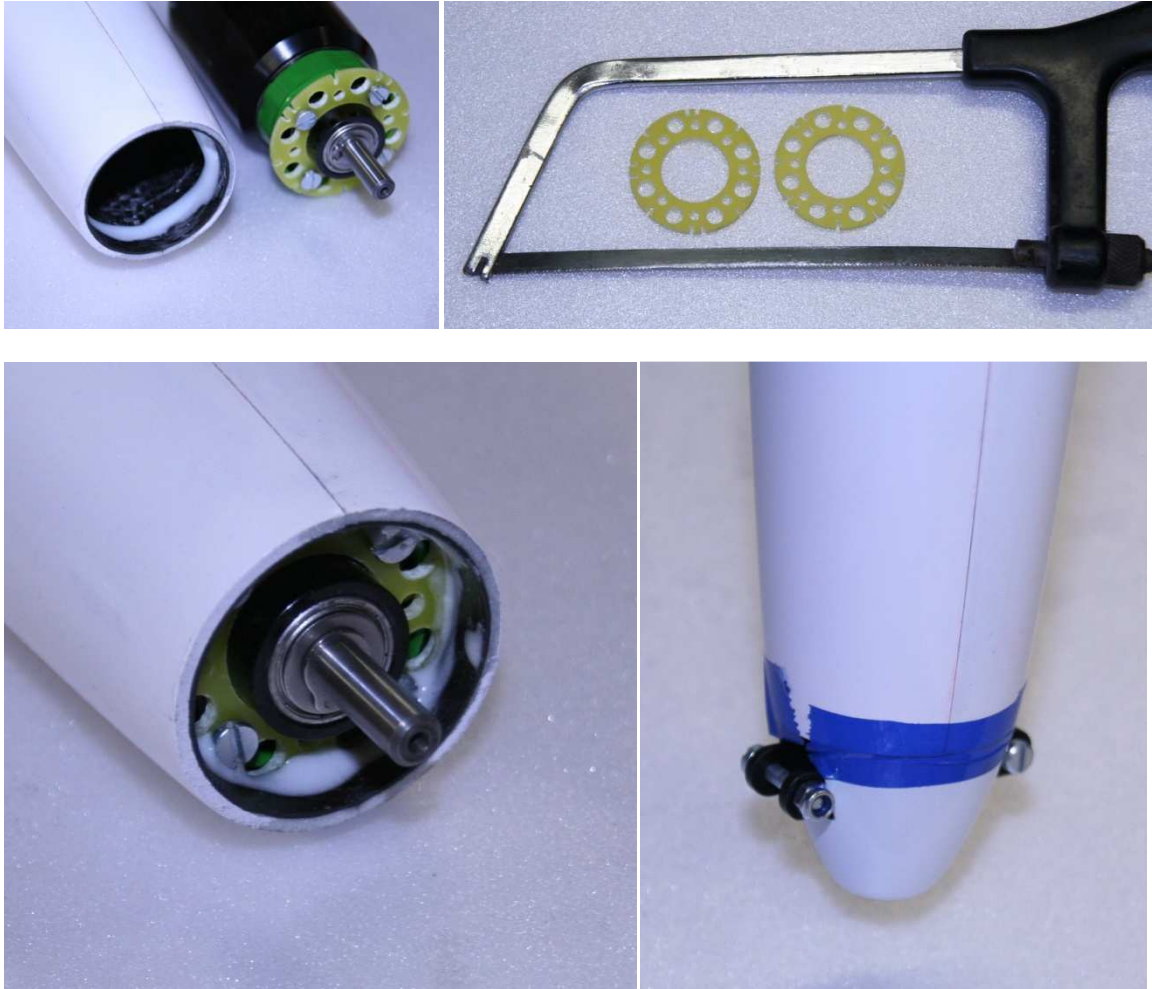
Picture 9: The glued-in of the engine-barrier
