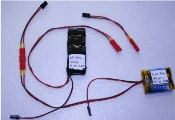
Picture 16: Voltage supplies for the deck equipment
