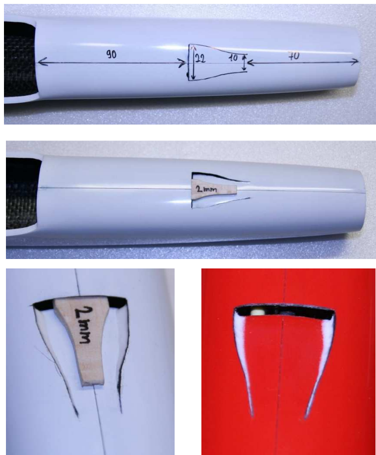
Picture 2: The cooling air's entrance
